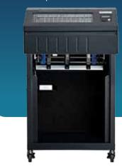
printed and serialized documents that require print on demand, single form tear-off usability. The Zero Tear is designed to eliminate wasted forms and reduce operating costs.
